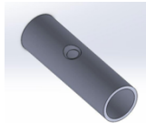
Figure 3: Design for 3D printed tube connector support with injection port
