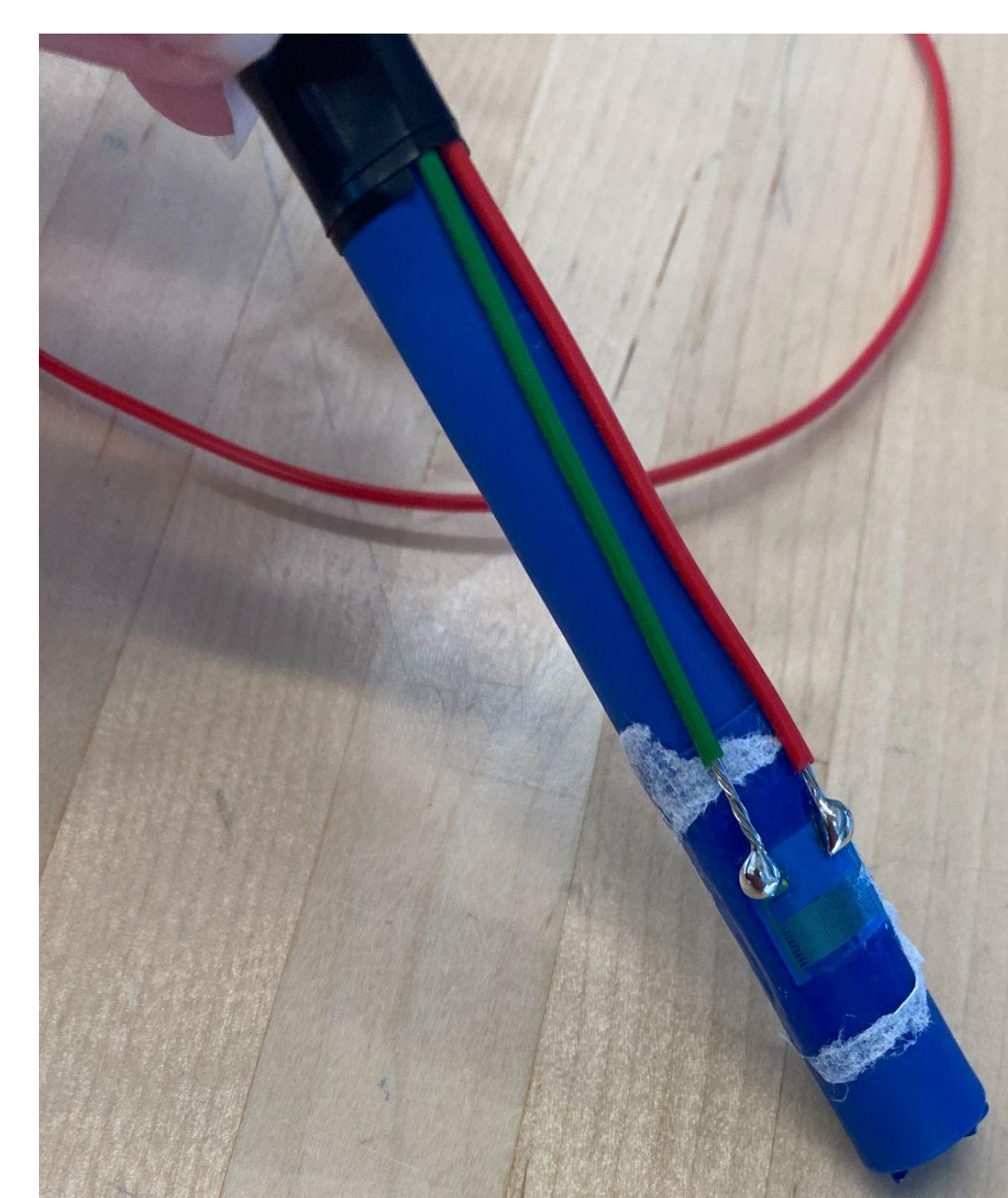
Figure 5 (below): Semiflexible interdigitated electrode attached to probe.
