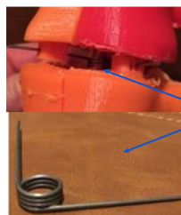
Figure 7: Torsional springs interconnect vertebrae and give appropriate relative rotation
