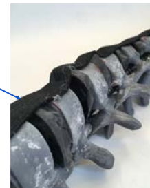
Figure 7: Torsional springs interconnect vertebrae and give appropriate relative rotation
