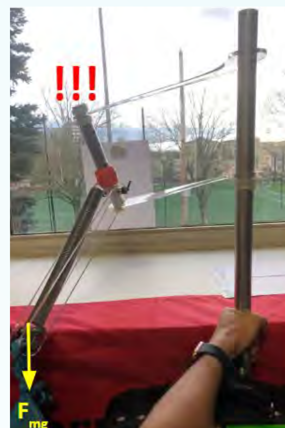
Figure G. Prototype 2 spring-load testing exhibits massive torsional stresses
