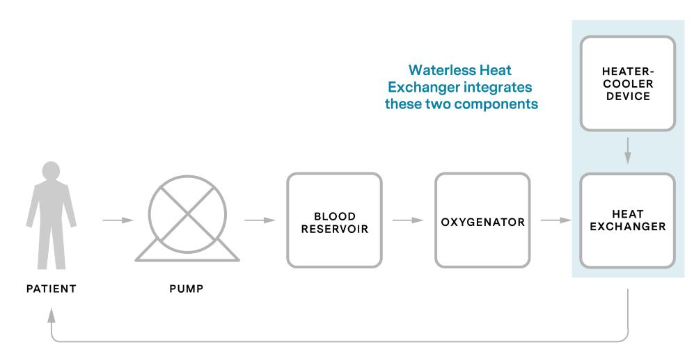
FIG 1. Overall Schematic of how an HCD works in conjunction with a CPB and how our device integrates with a CPB.
