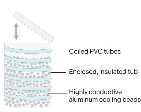
FIG 3. Cooling Unit Diagram.
