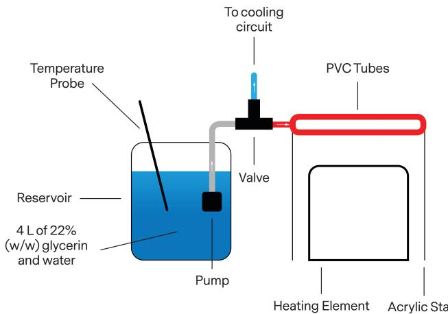
FIG 2. Heating Circuit Diagram.
