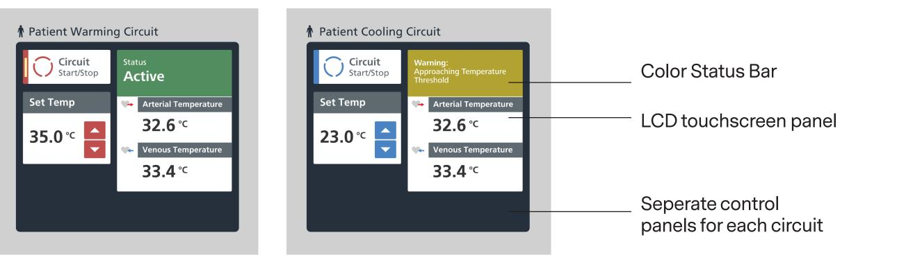
FIG 6. Control panel with normal status.
