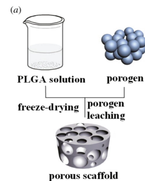
Figure 2: Methodology of creating porous PLGA scaffolds used as the inner capsule 3
