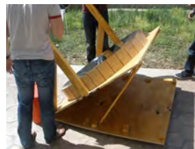
Figure 5: Mechanism for attaining specific pitch and rotation angle for maximum sunlight
