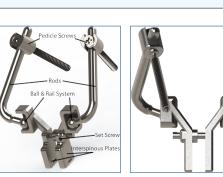
Figure 1 Isometric View of Design Rendered in Solidworks
