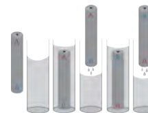
Figure 4: Dip coating method schematic
