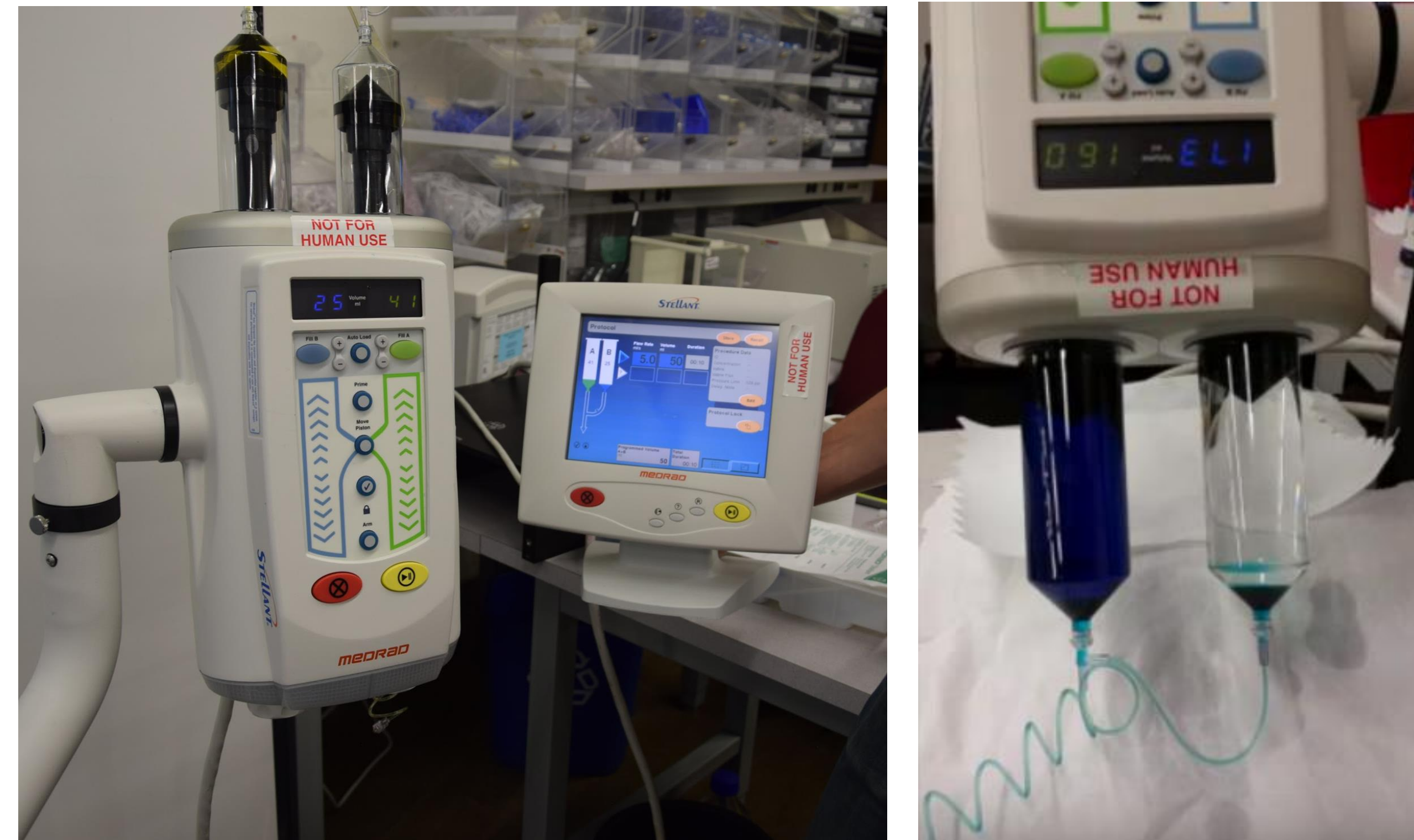
The above images show the current setup during an injection. The picture on the right was taken while the contrast (blue, left syringe) was being injected. This fluid can clearly be seen entering the saline syringe (clear, right syringe) and mixing.
