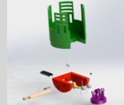
Figure 5. Illustrates an exploded view of prototype 3 featuring a ratcheted gear joint.
